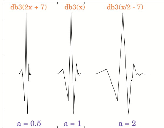
Figure 6-4: Time Scaled One-Dimensional Wavelet
